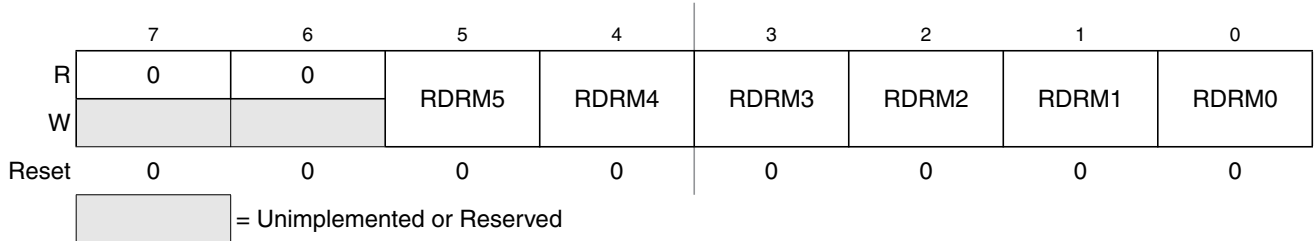
Figure 2-20. Port M Reduced Drive Register (RDRM)
